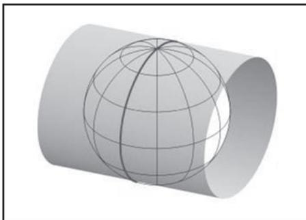
Figure 3. Transverse Mercator. The cylinder is tangent to the surface of the ellipsoid at a particular meridian of longitude. When points are projected onto the cylinder and the cylinder is unwrapped to a plane, distortions are minimized in the vicinity of this particular meridian.
