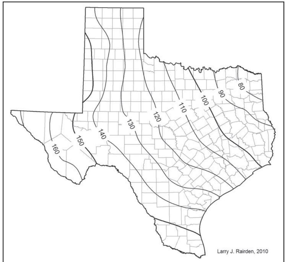
Figure 1. Magnitude of horizontal datum shift, in feet, between NAD27 and NAD83.
