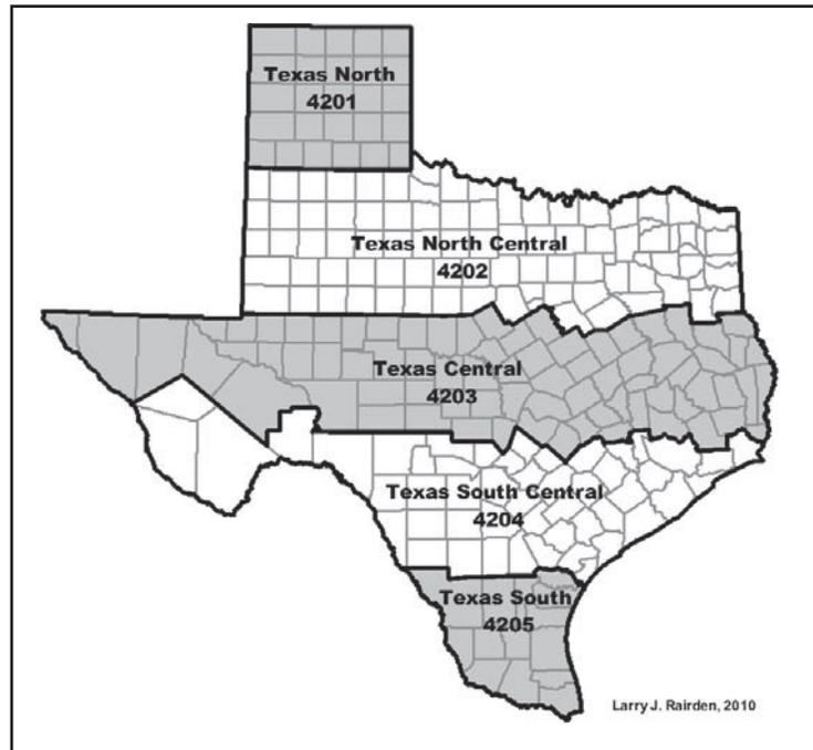
Figure 4. Texas is composed of five State Plane Coordinate System (SPCS) zones.
