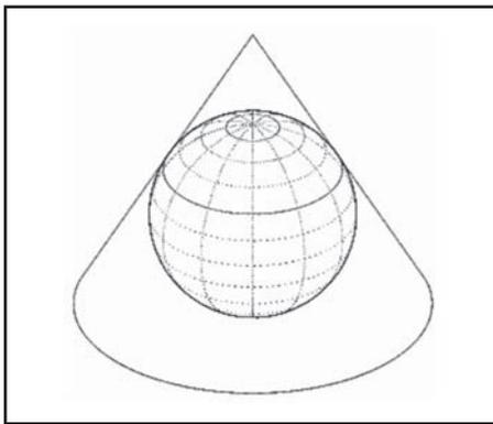
Figure 2. Lambert conformal conic. The cone is tangent to the surface of the ellipsoid at a particular latitude. When points are projected onto the cone and the cone is unwrapped to a plane, distortions are minimized in the vicinity of this particular latitude.
